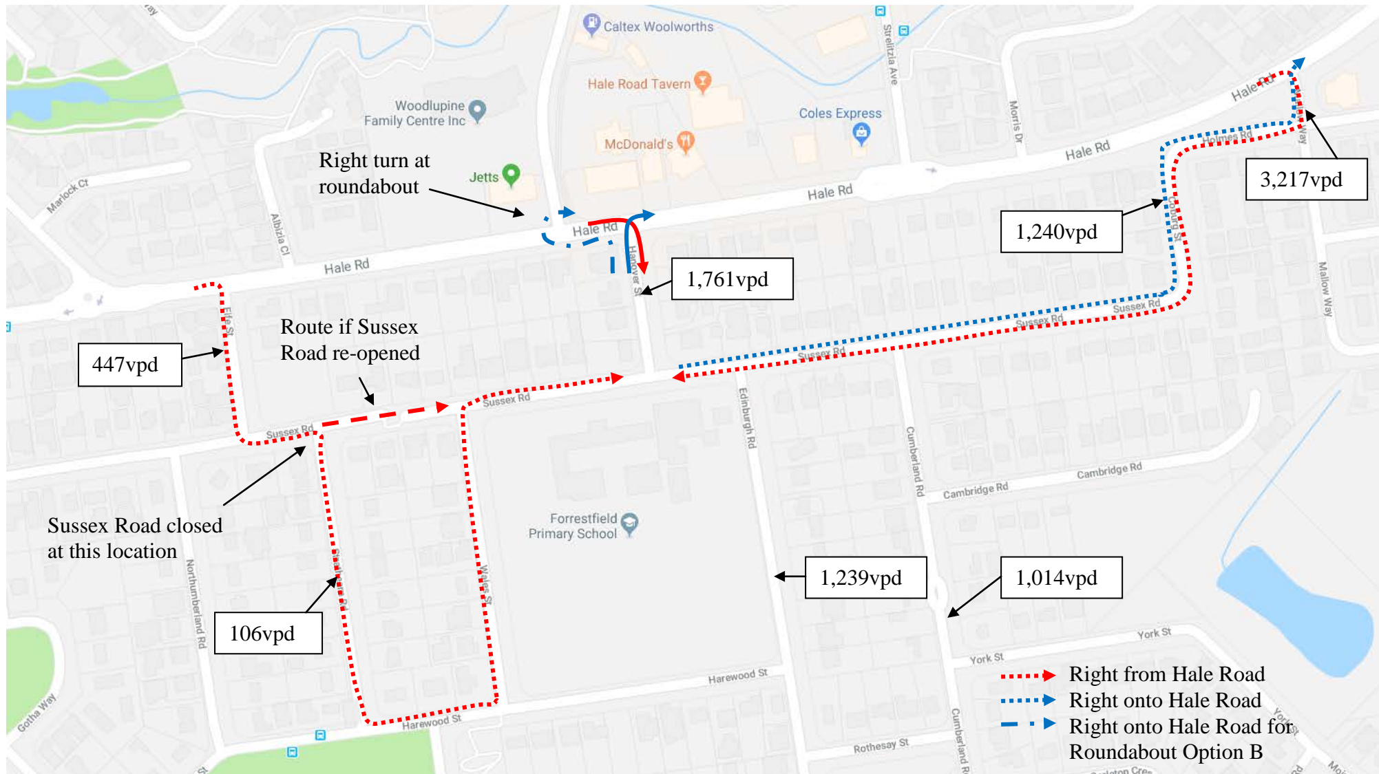
Figure 2: Alternative Routes with Hanover Street as left turns only including existing traffic volumes.
