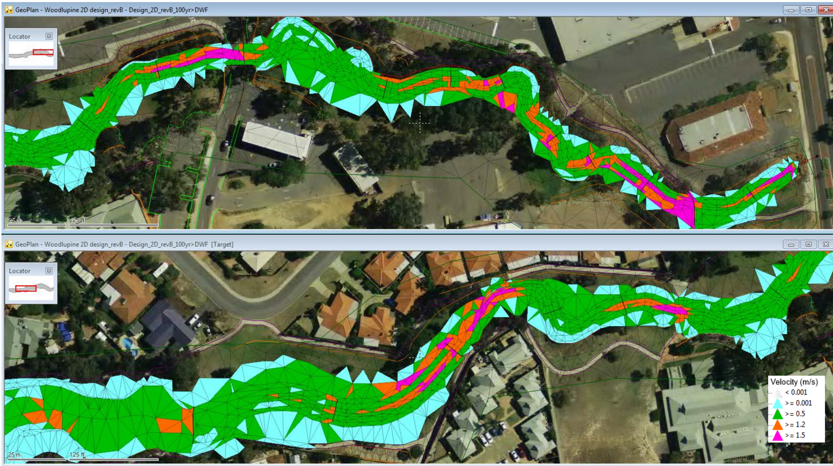
Figure 10: Concept design extent of flooding and velocities expected for major flood (100yr ARI)
