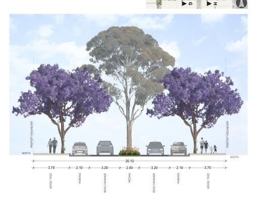
Figure 13: Section A-A Stirk Street (Corners)
