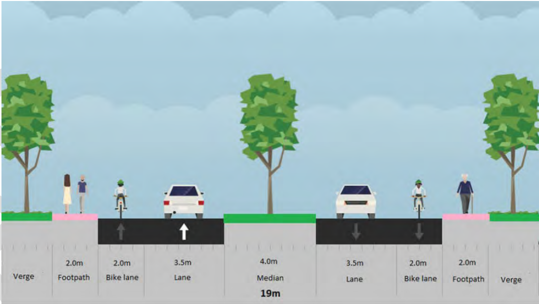
Figure 3-1 Typical Cross-section for a Low-Capacity Road
