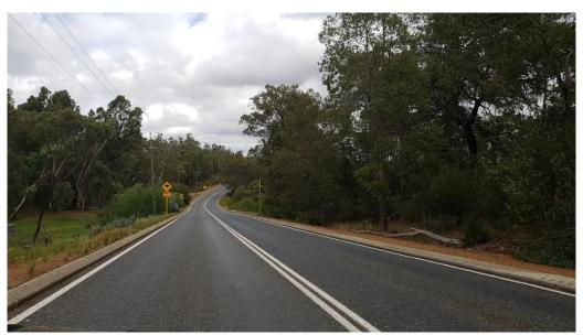
Photo 2: Typical combined horizontal and vertical curves within this section of Canning Road.
