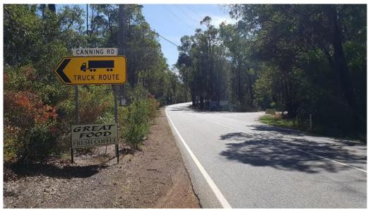
Photo 16: Intersection with an unnamed link road, looking north. Note lack of warning signs.
