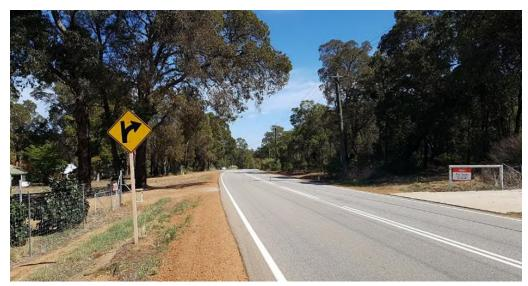
Photo 41: The warning sign does not fully identify the connections or potential movements.
