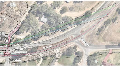
(SISD) SAFE INTERSECTION STOPPING DISTANCE PLAN 2
