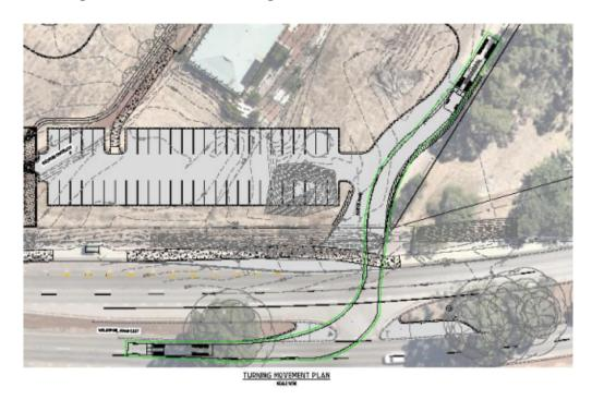
39. In order for 19m vehicles to make this turn in one movement, drivers need to have adequate sight distance – Safe Intersection Sight Distance (SSID) to their left (ie of vehicles coming from the east along Welshpool Rd East). A fully compliant design (for the posted 80 km/h speed limit plus 10 km/h as required in guidelines) would require SSID as shown in the following sketch:
