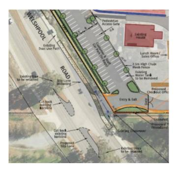
31. Turning Movement a) (from the west into driveway) is proposed to be facilitated by a deceleration 'slip' lane which also incorporates the existing embayed bus bay. This is shown in the following diagram:
