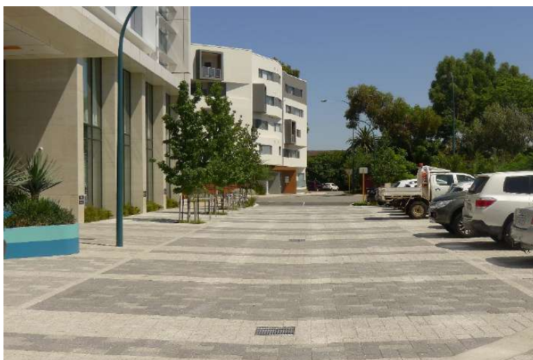
Plate 2: Permeable pavement with tree pits
