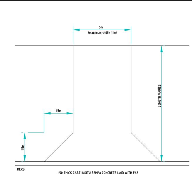
150 THICK CAST INSITU 32MPa CONCRETE LAID WITH F62 REINFORCEMENT 50mm FROM BOTTOM. CONCRETE TO BE LAID ON A COMPACTED SUBGRADE
