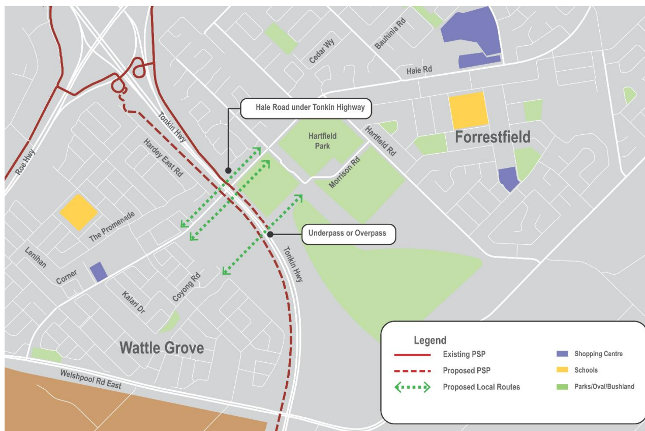
Figure 7-2 Tonkin Highway PSP – Recommended Arrangement
