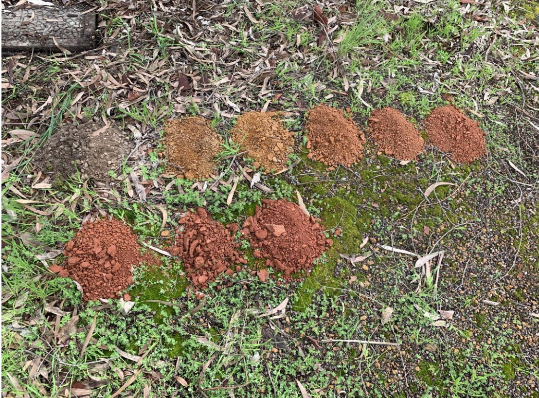
Figure 1: Samples collected at 0.5 m intervals during drilling
