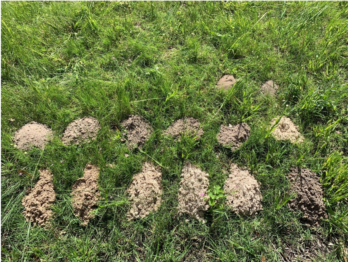
Figure 1: Samples collected at 0.5 m intervals during drilling
