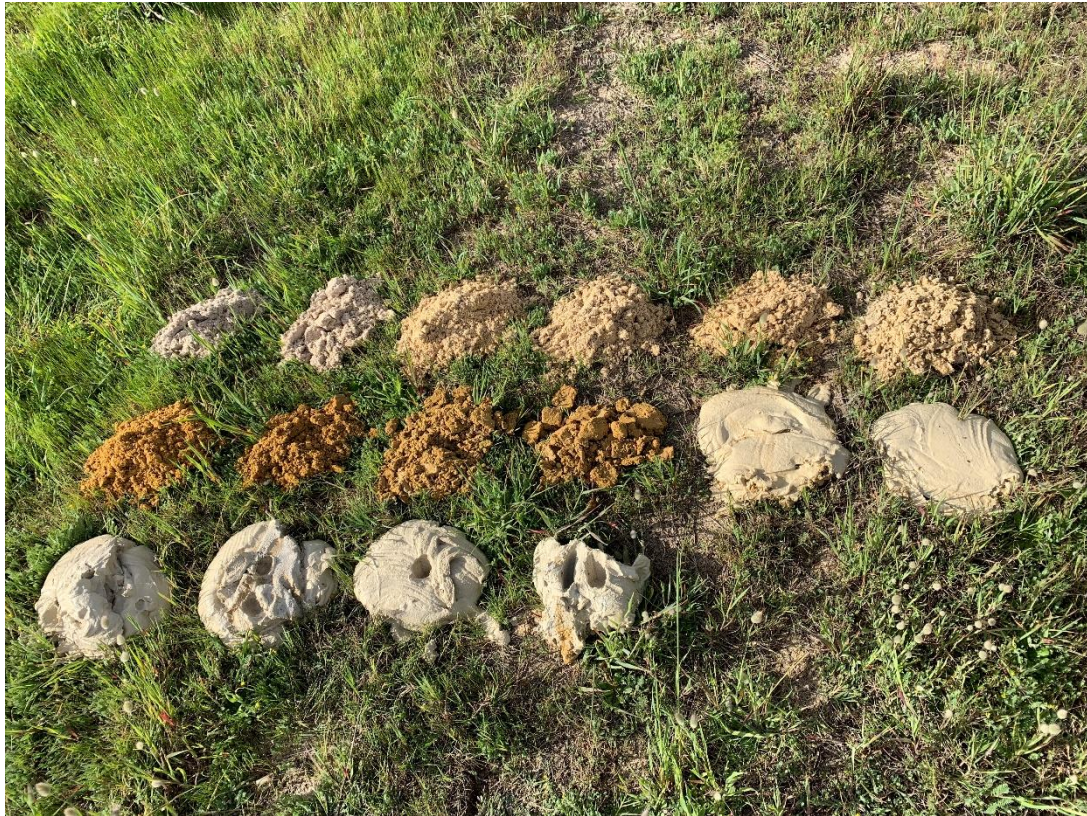
Figure 1: Samples collected at 0.5 m intervals during drilling
