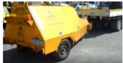
Falling Weight Deflectometer testing equipment
